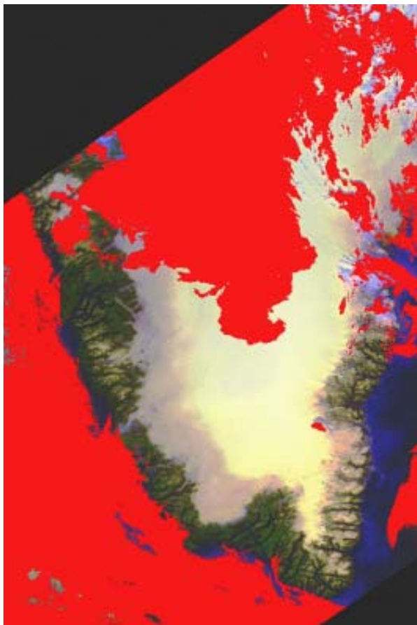
Figure 15.7. Example of a cloud mask (960718) calculated with default configuration values.
