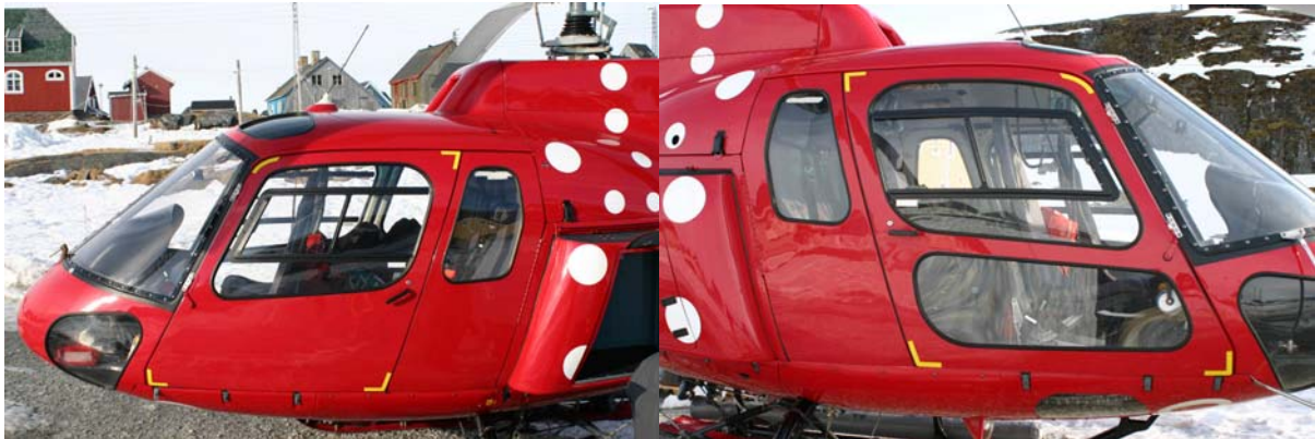
Figure 13. Window design on helicopter currently available for caribou surveys; left and right sides.
