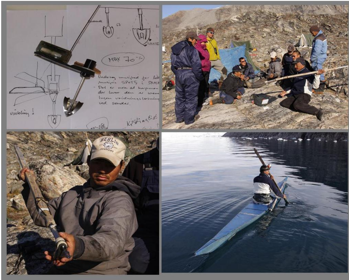
Photo 1. Satellite transmitter system for tagging narwhals in Melville Bay with harpoon mounting and approach in kayak.
