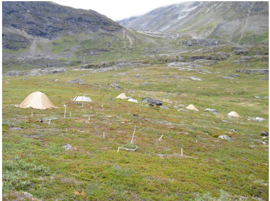
Figure 19. Overview of CO 2 flux plot site with Hessian tents for shadowing and ITEX hexagons for increasing temperature.
