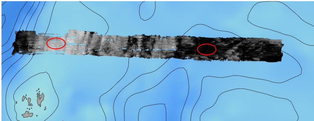
Figure 5. Example of raw backscatter mosaic generated on board showing bottom reflectivity as a manifestation of bottom hardness: lighter tones-stronger reflectivity-harder bottom. Red circles indicate recommended areas for ground-truthing that cover homogeneous tones of grayscales.
