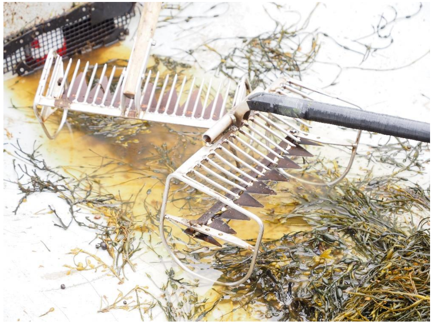
Figure 5.3. Seaweed harvester rake used by harvesters providing seaweed biomass for Acadian Seaplants Ltd.
