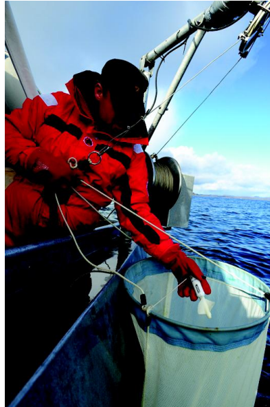
Fig. 8. Sampling with a 45- \mu\text{m} WP2-net equipped with a flow meter at the monthly samplings at Nuuk Ecological Research Operations. Photo L. Port.
