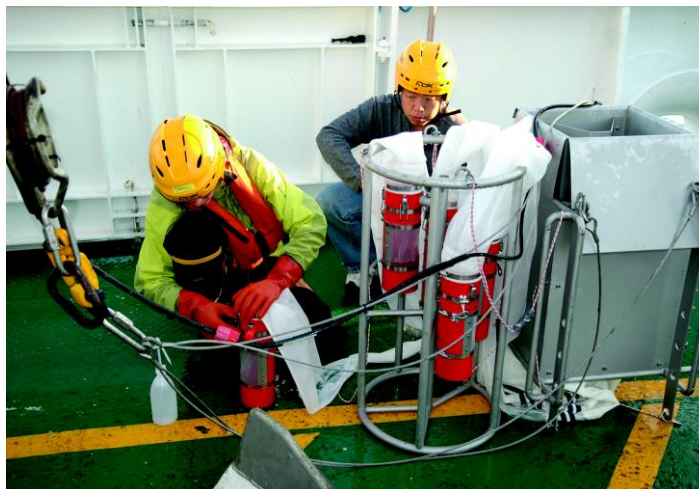
Fig. 7. Preparing for zooplankton sampling with a MultiNet ® equipped with five 50- \mu m nets. Photo S.H. Jónasdóttir.
