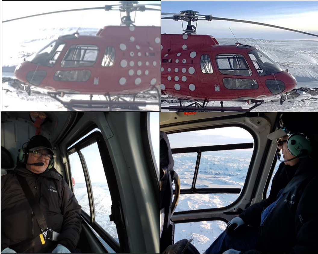
Figure 57. AS350 Helicopter viewing windows for the left and right sides, illustrating small rear window size and the numerous impediments obstructing viewing.
