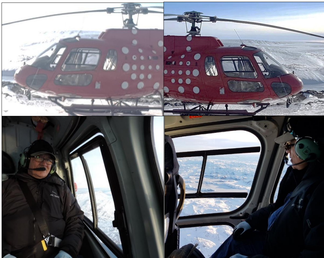
Figure 89. AS350 Helicopter viewing windows for the left and right sides, illustrating small rear window size and the numerous impediments obstructing viewing.
