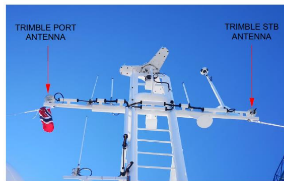
TRIMBLE ANTENNAE LOOKING FORWARD / UP
